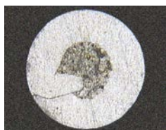
Elgacore® Matrix wire seam cross section ultra-consistent seam, smooth and tight.
